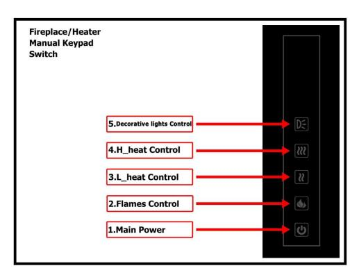
The first button on the control panel is the **(1) Main Power** button which is used to switch the appliance ON and OFF
